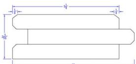
T&G Roof Decking - Deco Grade Lock Deck
