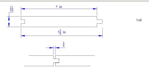
Vertical Grain T&G Patterns - Thermally Modified T&G Rev. Fineline RS/Finish Ready
