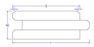
T&G Roof Decking - Deco Grade Lock Deck
